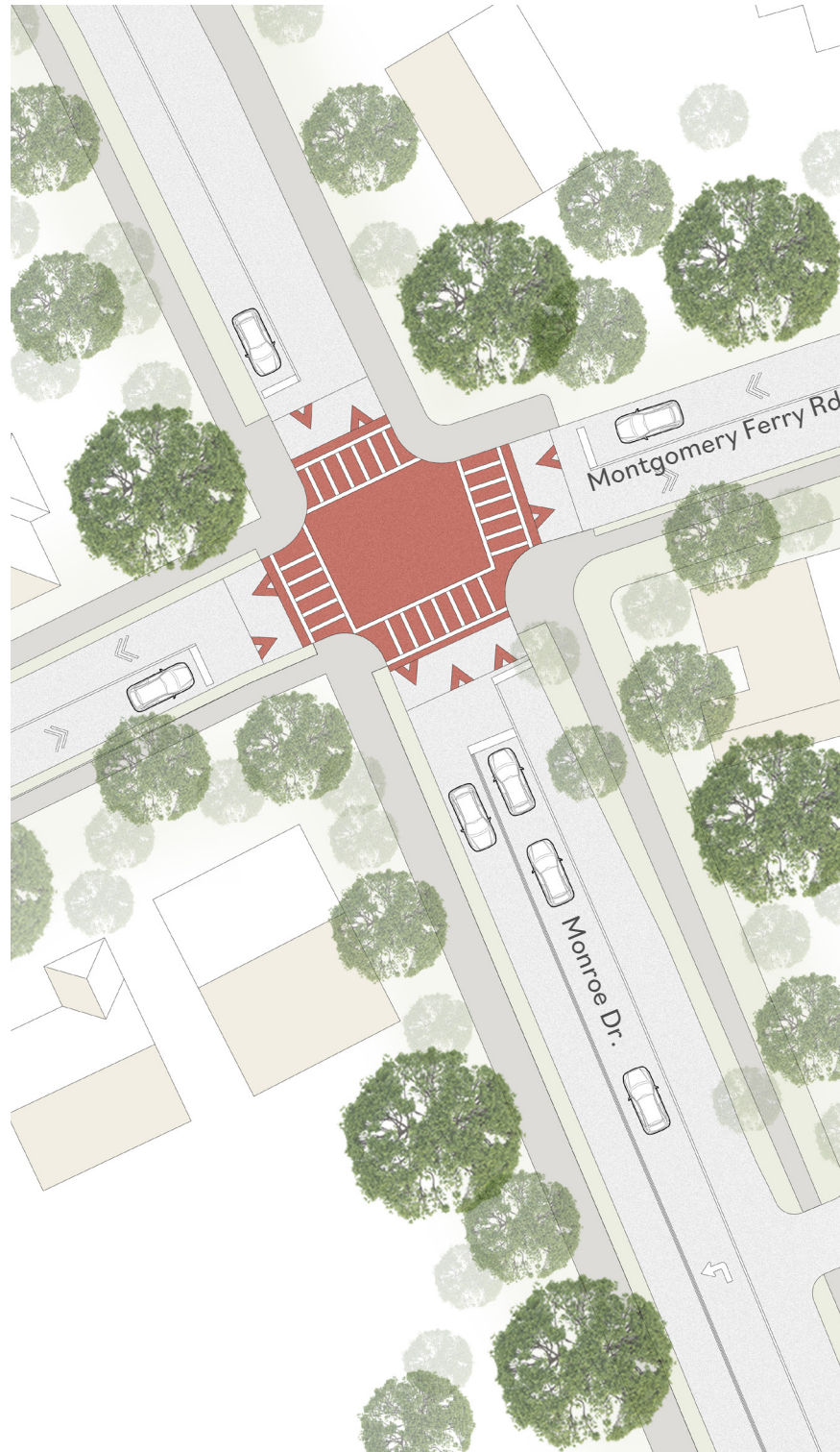
A speed table at the intersection of Montgomery Ferry Rd. and Monroe Dr. A speed table would not require curb readjustment as significant as with implementing a roundabout.
